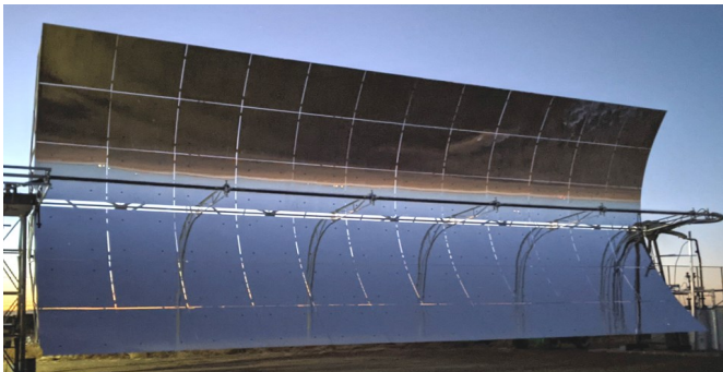
SunBeam™ Parabolic Trough Concentrator Full scale test module at Solar Dynamics test center
