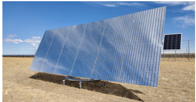
SunRing™ 27m² Wireless Heliostat Full scale test unit at Solar Dynamics test center
