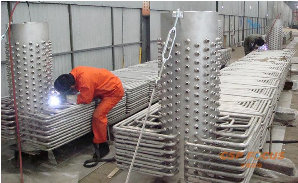
Figure 6-9 Example of Header / Coil Heat Exchanger Fabrication 44
