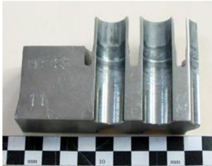
Figure 6-10 Example of an Internal Bore Welded Tube-to-Tubesheet Connection
