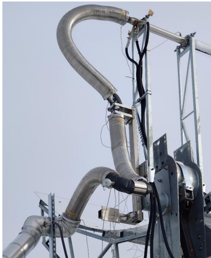
Figure 10-3 Flex Hose Assembly Installed on a Prototype Collector
